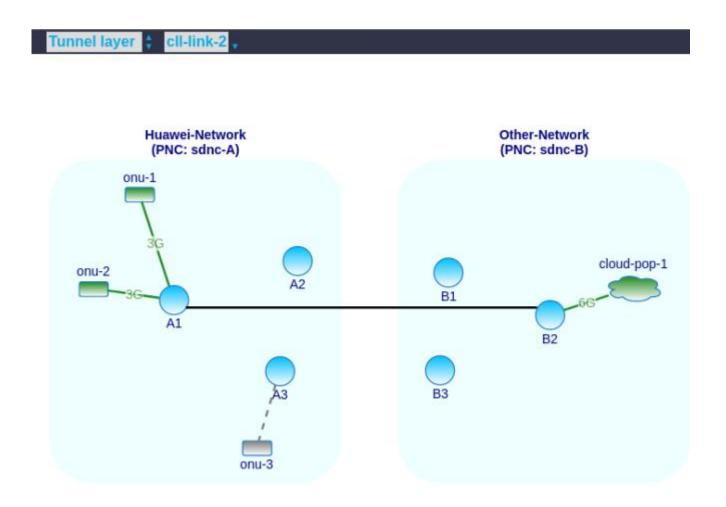
Tunnel layer view: displays installation and configuration for each OTN tunnel.
