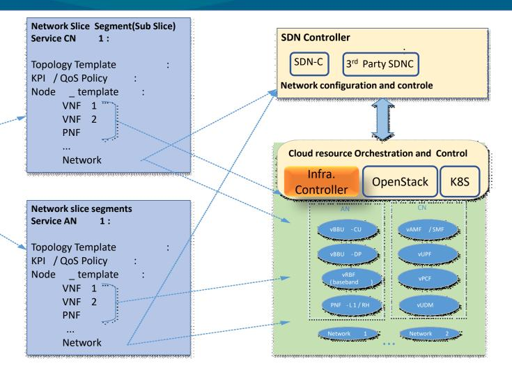
Nested service orchestration and Infrastructure controller is required to implement model-driven EtE slicing
