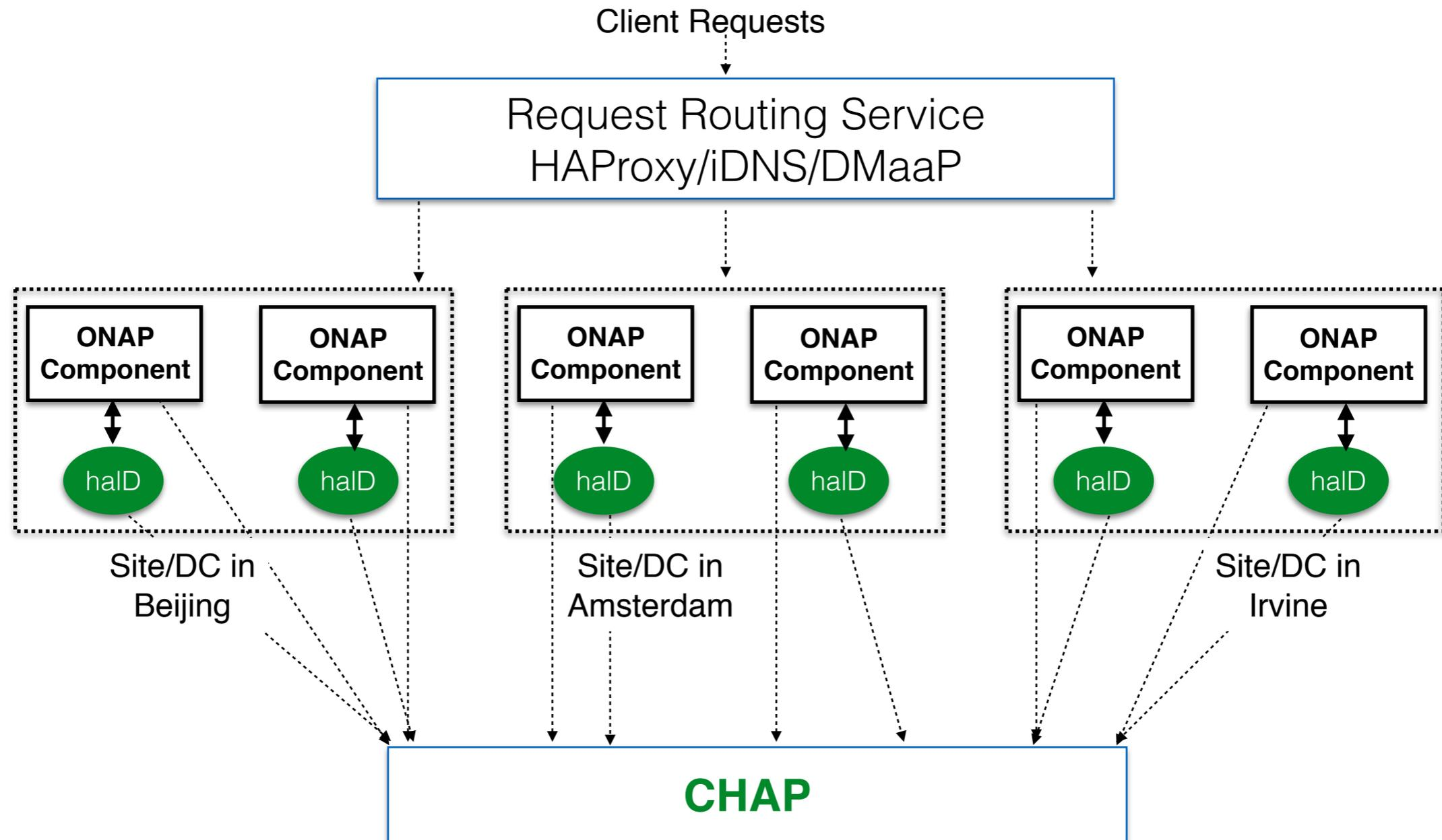
CHAP platform providing Conductor (distributed site selection service) that is used by the haDs and MUSIC (distributed multi-site state management service) that is used by both the haDs and ONAP components
