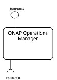
Definition: OOM is the life cycle manager of the ONAP platform (i.e. SDC, SO, SDNC, etc.). OOM uses the Kubernetes container management system and Consul to provide the following functionality:
