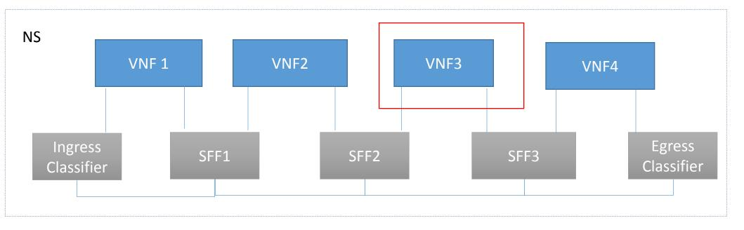
One or more of the VNF in a service chain is marked for maintenance
