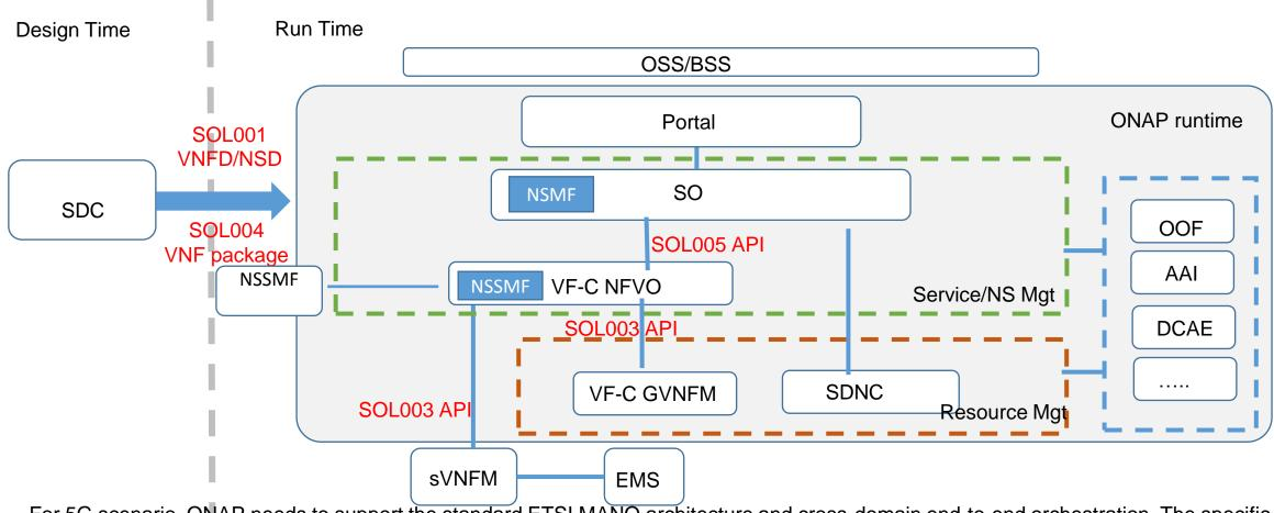
For 5G scenario, ONAP needs to support the standard ETSI MANO architecture and cross-domain end-to-end orchestration. The specific requirements for ONAP in this scenario:
