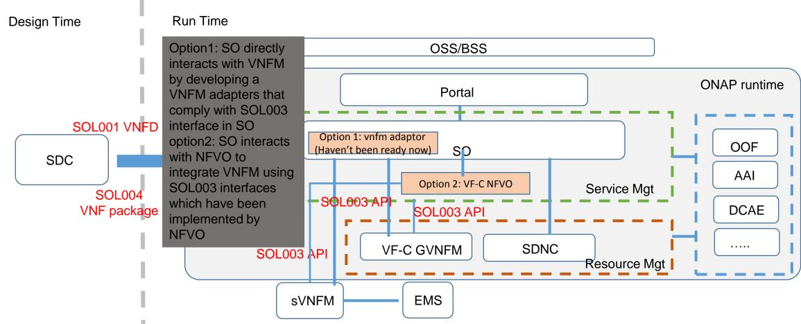
For vCPE deployment based on standard VNFD, ONAP needs to support the standard VNFD and cross-domain orchestration and doesn't need to support standard NS. The specific requirements for ONAP in this scenario:
