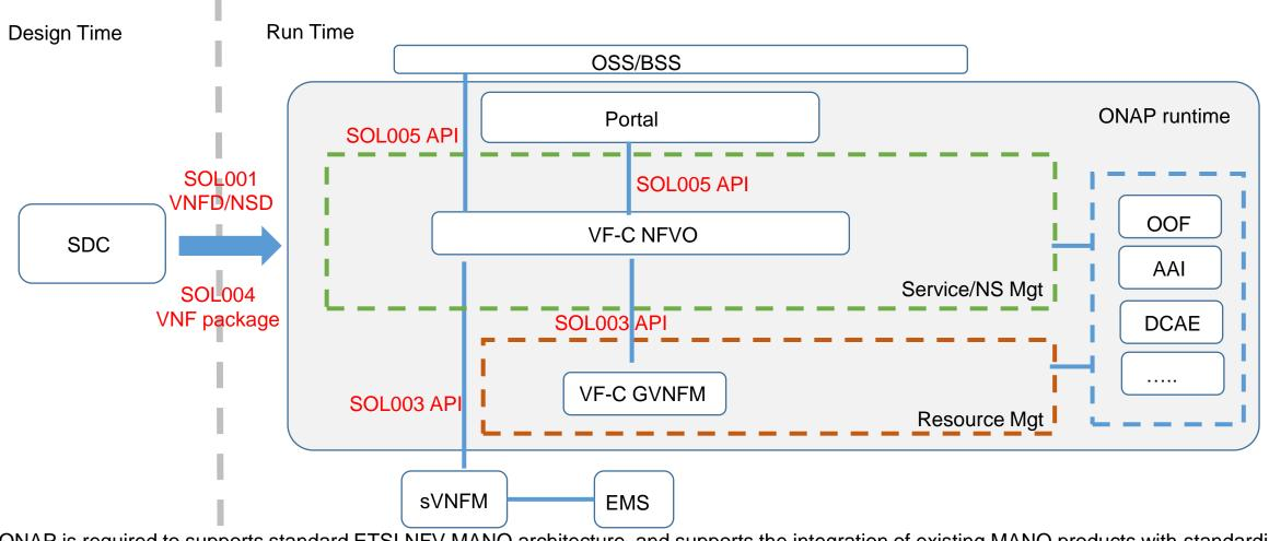
ONAP is required to supports standard ETSI NFV MANO architecture, and supports the integration of existing MANO products with standardized models and interfaces. It also facilitates operators to incubate self-developed MANO products. The specific requirements for ONAP in this scenario:
