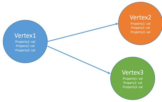
The adjacency list of a vertex contains all of the vertex's incident edges (and properties).
