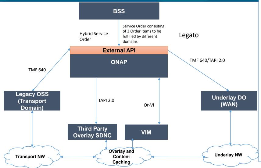
Current Implementation: Any end to end hybrid service request (received by External API as Service Order) should be processed by SO and then delegated to ONAP SDNC for resource activation and configuration, VF-C/App-C, Multi- VIM for VNF Orchestration. ONAP SDNC interacts with all the related network controllers to realize the activation request.
