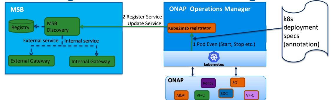
Kube2msb registrator can register service endpoints for the microservices deployed by OOM
