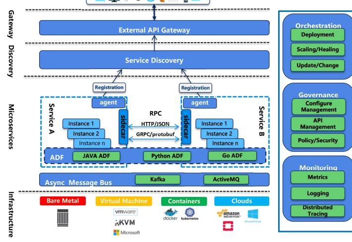
**OMSA** is the vision of ONAP Microservice Architecture to support carrier-grade requirements of ONAP microservices, which includes service registration/discovery, service communication, API gateway, service orchestration, service governance and service monitoring, etc.
