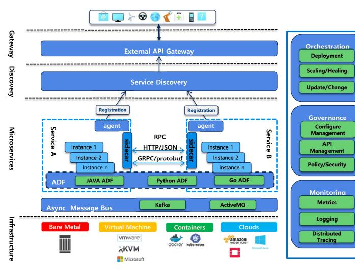
**OMSA** is the vision of ONAP Microservice Architecture to support carrier-grade requirements of ONAP microservices, which includes service registration/discovery, service communication, API gateway, service orchestration, service governance and service monitoring, etc.
