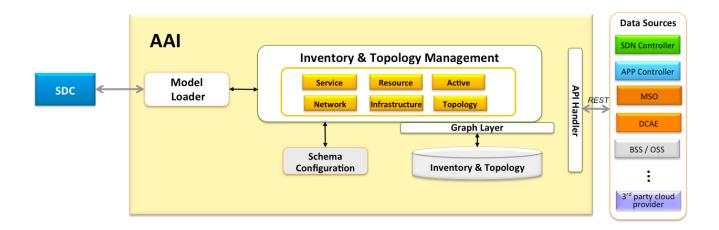
Figure 1. Active and Available Inventory (AAI) functional diagram
