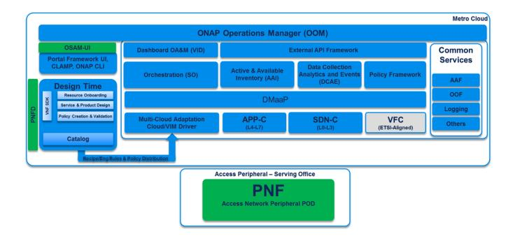
OSAM use case will use the similar approach to 5g use-case. OSAM consists of three components which are OSAM Gateway, OSAM Core, and SEBA. OSAM Gateway and OSAM Core and SEBA will be onboard as a service to ONAP.
