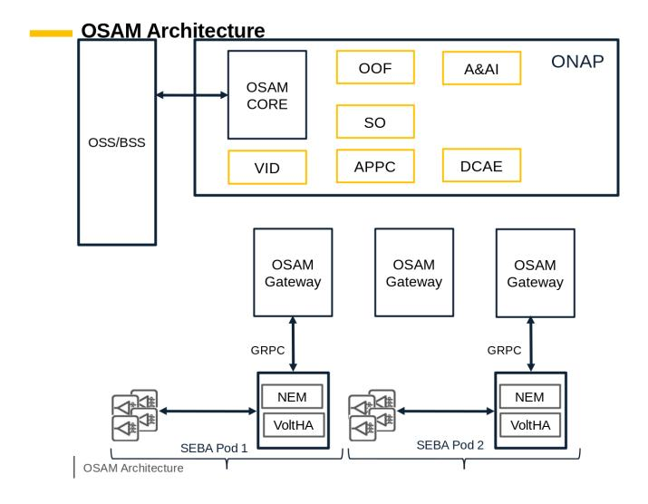
OSAM is addressed as PNF model of 5G use case. In 5G use case, CU and DU pairs are used. In our OSAM case, we are going to use the similar approach. SEBA is going to be mapped as DU. OSAM GW(Gateway) is going to be mapped as CU.
