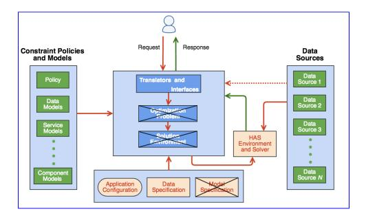
The HAS application highlights how a custom optimization application can utilize the OOF. In this specific case, the HAS application provides on its own: (a) an execution environment, (b) an API specification, (c) adapters to data components such as A&AI and SO, (d) and a custom optimization algorithm /solver. The HAS application relies on OOF for policy retrieval and translation.
