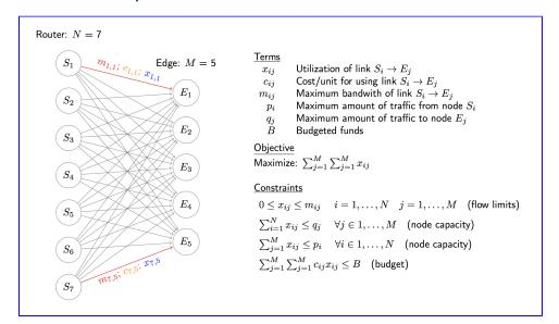
Illustration of the budget-constrained max-flow problem. Given a set of starting nodes and destination nodes, the objective is to calculate the maximum amount of "flow" across the nodes, subject to capacity constraints of nodes, constraints on the capacity of the connections (edges), as well as costs associated with utilization of each connection (edge). The objective is to maximize the flow subject to the budget constraint.
