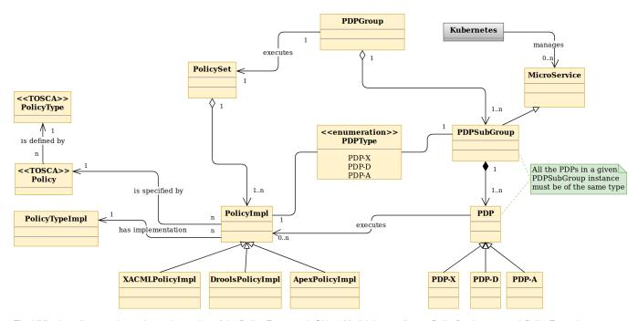
The UML class diagram above shows the portion of the Policy Framework Object Model that applies to PolicyDeployment and PolicyExecution.
