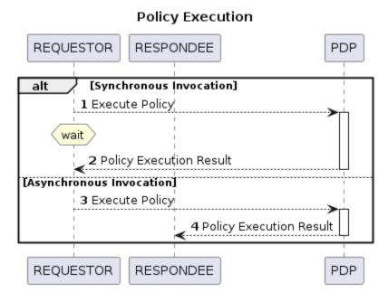
Policy execution can be synchronous or asynchronous. In synchronous policy execution, the component requesting a policy decision requests a policy decision and waits for the result. The PDP-X and PDP-A use synchronous policy execution. In asynchronous policy execution, the component that requests a policy decision does not wait for the decision. Indeed, the decision may be passed to another component. The PDP-D and PDP-A use asynchronous policy execution.
