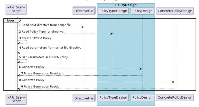
One straightforward way of generating policies from Policy types is to use directives specified in a script file. The command line utility is an *API\_User*. The script reads directives from a file. For each directive, it reads the policy type using the Policy Type API, and uses the parameters of the directive to create a TOSCA Policy. It then uses the Policy API to create the policy.
