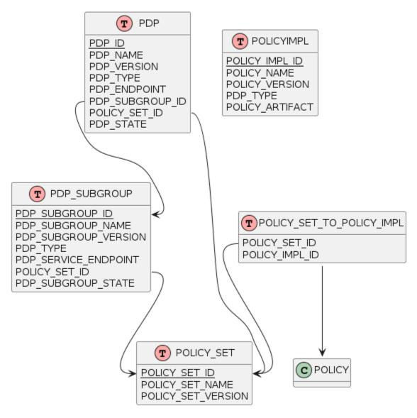
The diagram above gives an indicative structure of the run time topology information in the Policy Framework database. Note that the *PDP\_SUBGROUP\_S TATE* and *PDP\_STATE* fields hold state information for life cycle management of PDP groups and PDPs.
