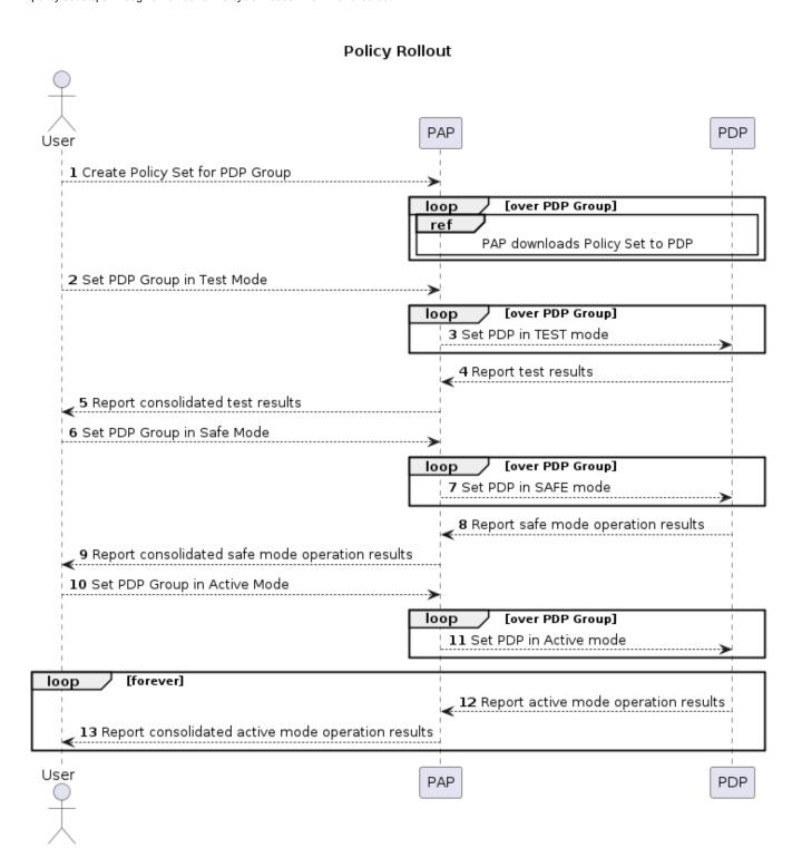
The user defines the set of policies for a PDP group. It is deployed to a PDP group and is initially in PASSIVE mode. The user sets the PDP Group into TEST mode. The policies are run in a test or sandboxed environment for a period of time. The test results are passed back to the user. The user may revert the policy set to PASSIVE mode a number of times and upgrade the policy set during test operation.
