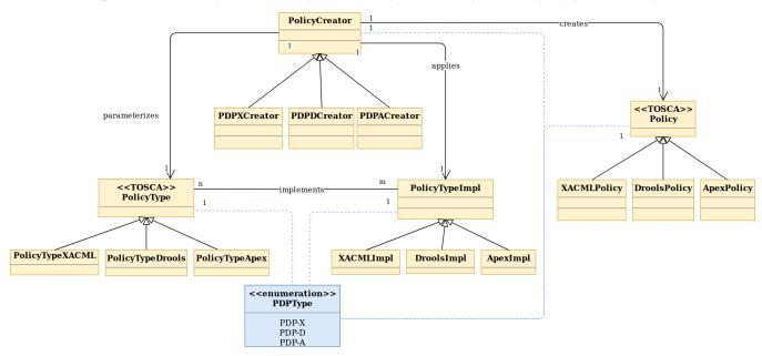
The UML class diagram above shows the portion of the Policy Framework Object Model that applies to PolicyDevelopment and PolicyDeployment.
