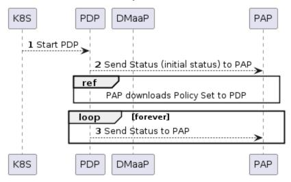
At startup, the PDP initializes itself. At this point it is in PASSIVE mode. The PDP begins sending periodic Status messages to the PAP.
