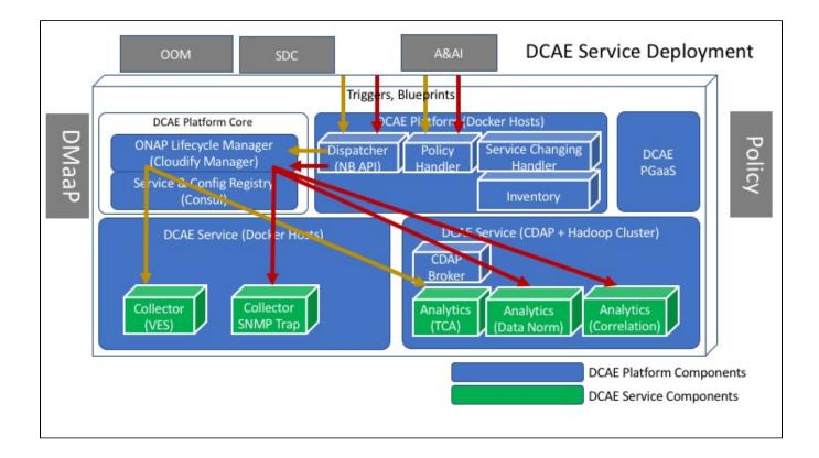
The figure below further illustrates how performance measurement and fault management data, i.e. VNF events, SNMP traps, and alert events, traverse through the DCAE Service components, and eventually depart from DCAE to reach downstream components such as ONAP Policy, or other external systems such as ticketing.
