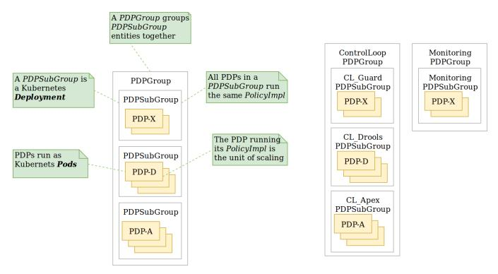
In order to achieve horizontal scalability, we group the PDPs running instances of a given *PolicyImpl* entity logically together into a *PDPSubGroup*. The number of PDPs in a *PDPSubGroup* can then be scaled up and down using Kubernetes. In other words, all PDPs in a subgroup run the same *PolicyImpl*, that is the same policy template implementation (in XACML, Drools, or APEX) with the same parameters.
