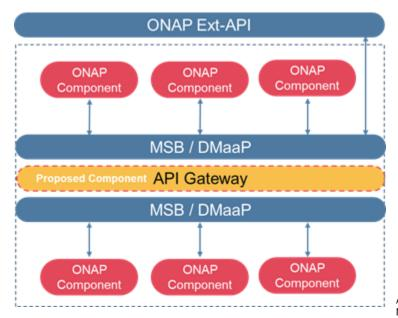
API GW closely works with three components in ONAP – Ext-API, MSB and DMaaP. API GW can provide a proxy interface to Ext-API
